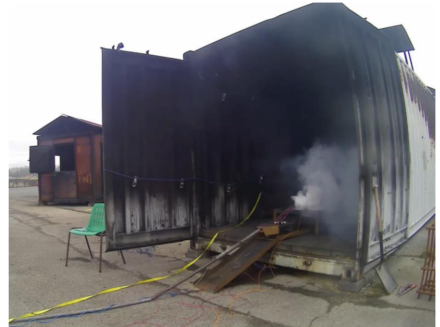
Vapour cloud from 1.7 kWh LiB module at 50% SoC i.e. a VAPOUR CLOUD
